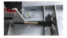
This unit is equipped with two 16,000 lb. leveling ratchet jacks.
